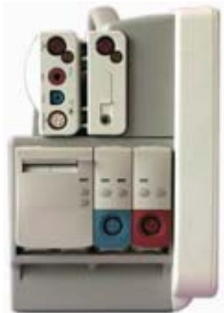
Side view of MP40/MP50 with MMS and MMS extension (top), and plug-in recorder module and two measurement modules below
